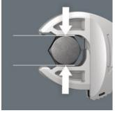
The parallel smooth jaws of the Joker 6004 allow surface pressure and can thus prevent rounding of the bolt or screw head, which can occur during power transmission via the corners.
