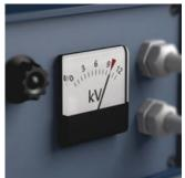
Each Kraftform Kompakt VDE set has been tested individually at 10,000 volts, in accordance with IEC 60900.This ten-times-higher testing load guarantees safe working at their maximum permitted load of 1,000 volts.
