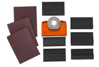
Consisting of 1 holder and 6 different profiles: 1 V-form for 90° angle, 1 trapezium for tongue-and-groove connections, 1 for straight profiles, 1 for convex forms (large), 1 each for concave and convex forms (small), as well as 5 sanding sheets grit 80, 120, and 180.
